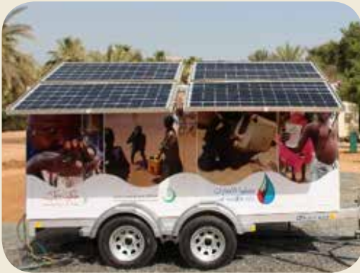
A portable Photovoltaic Reverse Osmosis (PVRO) unit operated by solar panels, which has a water production capacity of 7.7 m 3 /day.
