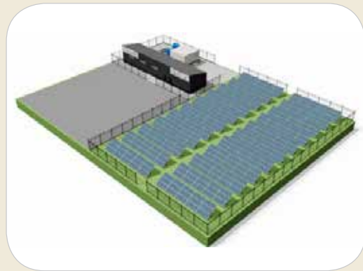
A larger scale, solar panel powered PVRO unit with storage and a production capacity of 50 m 3 /day.
